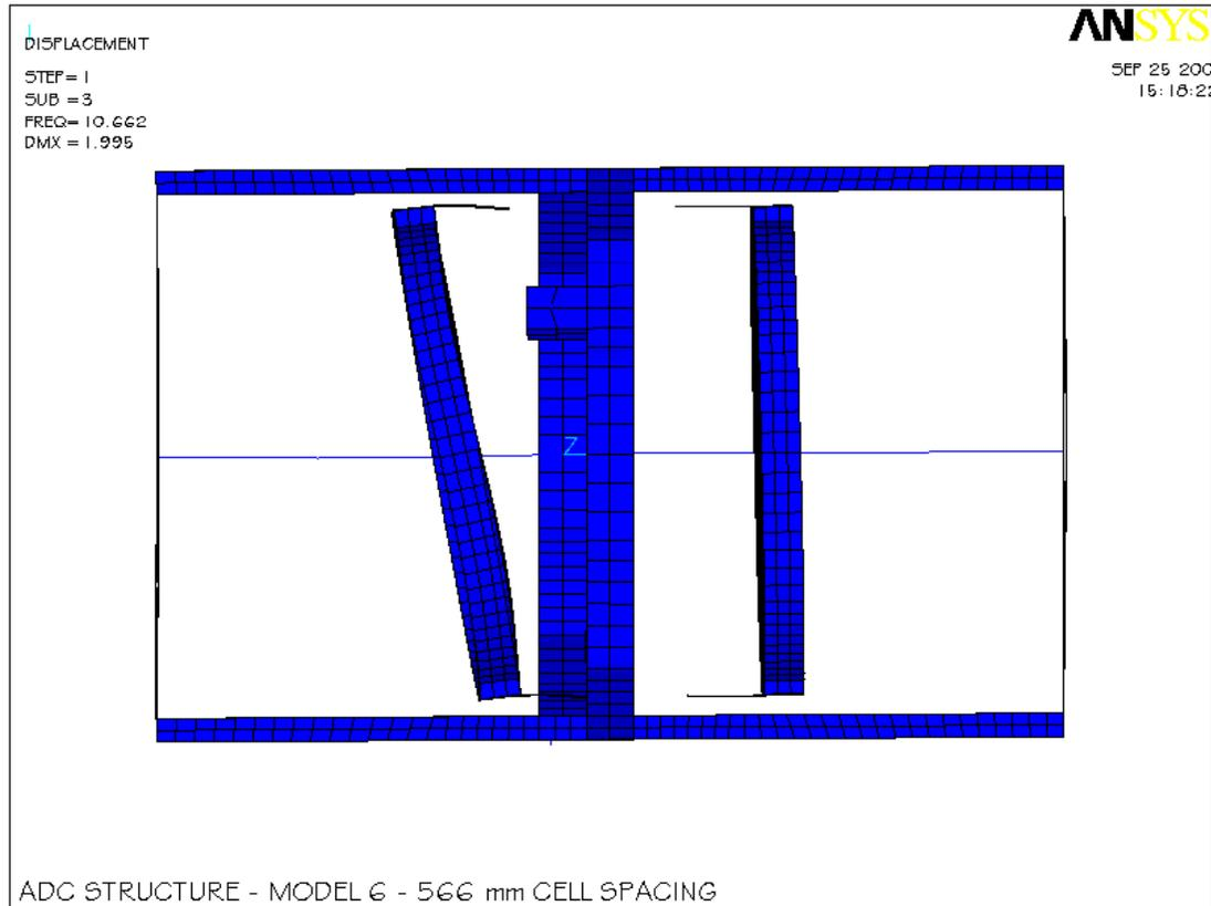
Figure 4.8 Mode #3, 10.7 hertz, theta y rotation of aft cell.
